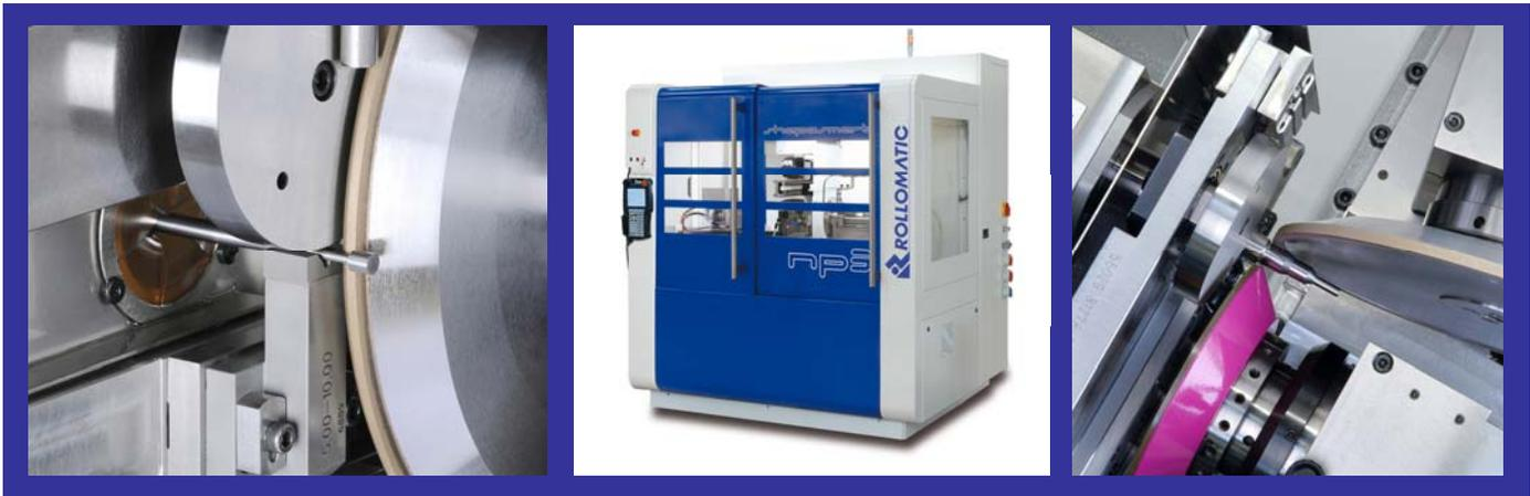
The peel or pinch/peel grinding method well proven on other types of the ShapeSmart® series provides the ability to grind tools with extreme length /diameter ratio as well as complex profiles. In addition, the rigid design of this machine equipped with a powerful 8.5 kW spindle motor and a wheel diameter of 250 mm (10") allows grinding parts requiring high material removal.
