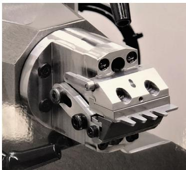
Clamping of a woodworking profile blade
