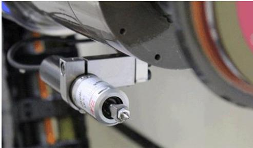
Prior to starting the grinding process, the exact position of the workpiece is determined using a 3D touch probe. Upon completion of the treatment, the device is also used to control vital geometrical characteristics of the workpiece (Photo: Klaus Vollrath)
