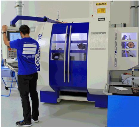
The five-axis model 529XW is suitable for producing precision cutting tools with diameters between 1 and 20 mm. The automatic system for the exchange of grinding wheel sets is docked at the right-hand side (Photo: Klaus Vollrath)
