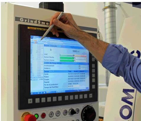
The control system can be easily and quickly programmed using a tracer pin (Photo: Klaus Vollrath)
