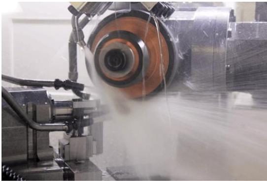
The oil used to cool and lubricate the workpiece and grinding wheel is very carefully filtered and tempered (Photo: Klaus Vollrath)
