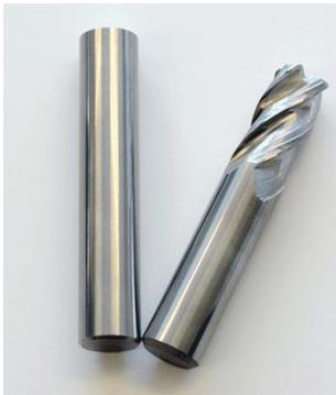
The production of this cylindrical milling tool from a blank with a diameter of 20 mm takes only about a quarter of an hour (Photo: Rollomatic)
