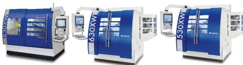
ShapeSmart 4/5-axis CNC pinch and peel grinding machines
