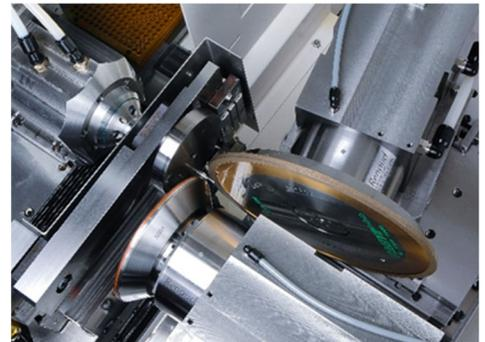
Carbide and steel pins, long and thin, ground on the Rollomatic ShapeSmart pinch/peel grinder for these industries:
