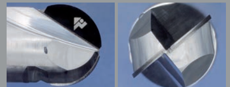
Tool: Ball nose endmill \varnothing 12 mm, 2 teeth Material: CVD, thickness 0.5 mm Operations: Primary, secondary relief angles Cycle time: 12 min
