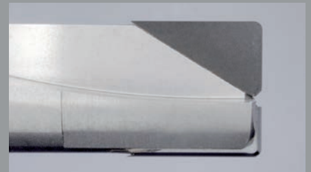
Tool: Endmill \varnothing 8, r 0.5, 2 teeth Material: PCD, thickness 1.6 mm Operations: Primary, secondary relief angles Cycle time: 26 min
