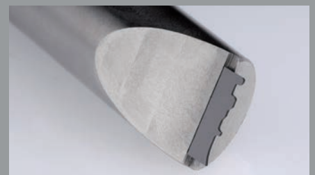
Special tool Material: CVD, thickness 0.5 mm length: 10 mm Operations: Primary, secondary relief angles Cycle time: 12 min
