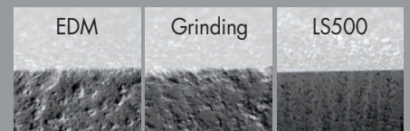
Cutting edge comparison with alternate process, magnified x 1000
